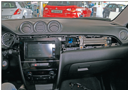
4. Suzuki Vitara dash board after removing center panel
